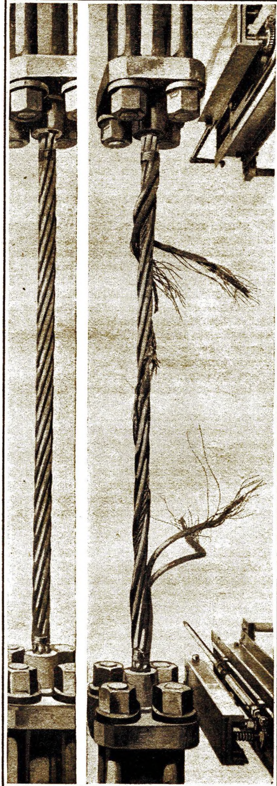
WIRE ROPE, BEFORE AND AFTER BEING TESTED. IT IS PROBABLE THAT NO COMMERCIAL STEEL CABLE HAS EVER BEEN BUILT WHICH COULD LONG WITHSTAND THE MIGHTY TUG OF UNCLE SAM'S GREAT ENGINES.
